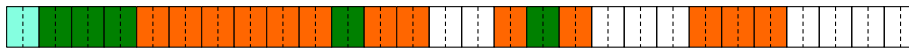
Figure 5: A cluster can be seen visually as an array. In this image, for example, we've shown three types of cluster: metadata fixed position (azure), metadata variable position (green), file data (orange), unused space (white).
