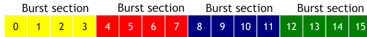
Figure 30: In the figure, a 16-byte address space is divided into 4-byte burst sections. In practice, address spaces are much larger (e.g., 4 GB) and burst sections are also larger (e.g., 128 bytes or more).
